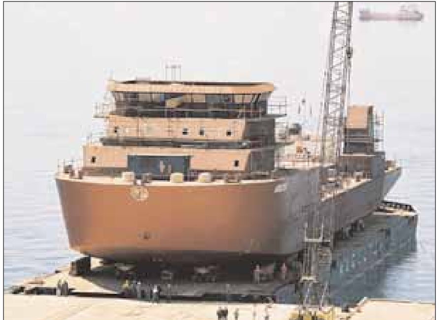
Above: The 'Arcos' being transferred from the 84 axle SPMT onto concrete blocks mounted on top of the barge.
